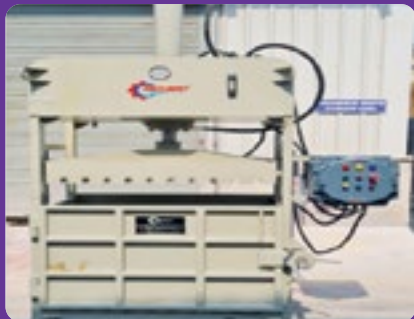
Bale press compacting for RM bags
